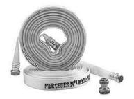
Mertex® is a circular woven hose with an extruded inner lining of thermoplastic polyurethane (TPU). The hose is very lightweight yet rugged with good mechanical properties. Mertex® performs excellent under all climatic conditions from -50  $^{\circ}$ C to +75  $^{\circ}$ C. Intermittent use up to +80  $^{\circ}$ C.
