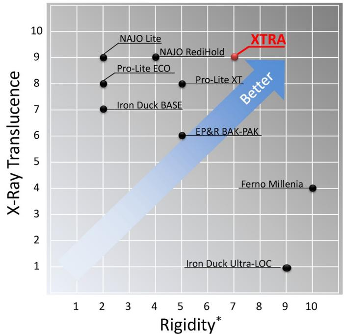
\*Rigidity specification based upon the deflection from horizontal of the center of the backboard with a 400 lb. distributed load, backboard supported at each end.
